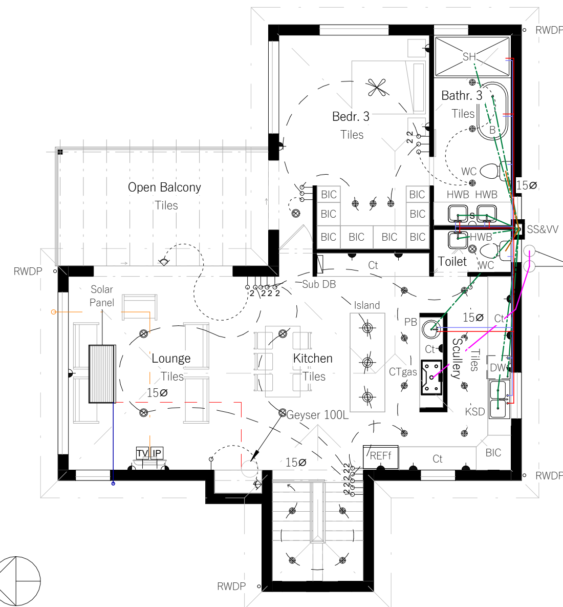
01 -First Storey Plumbing & Electrical Plan 1 : 100
